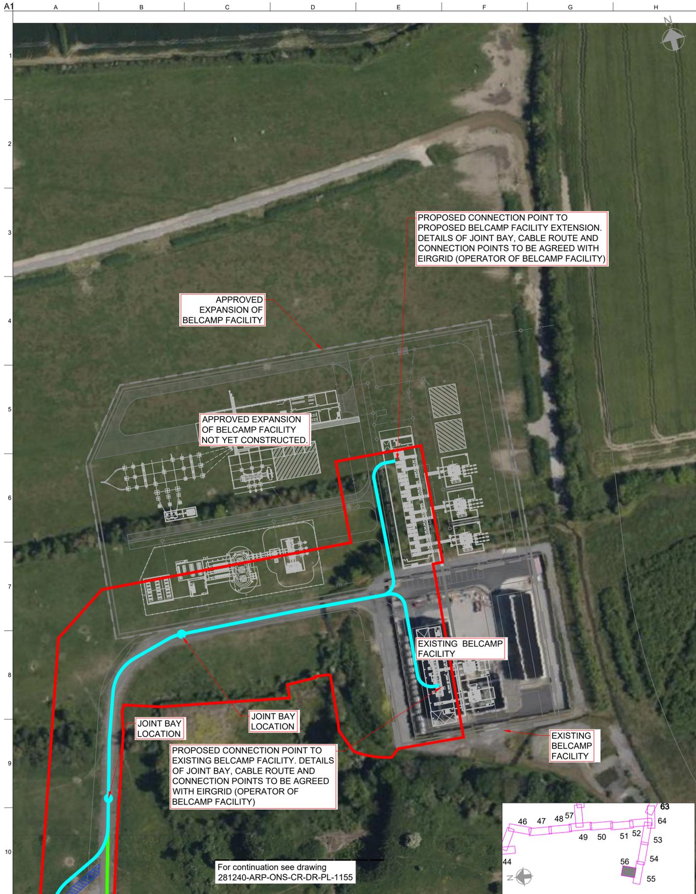
PROPOSED CONNECTION POINT TO PROPOSED BELCAMP FACILITY EXTENSION. DETAILS OF JOINT BAY, CABLE ROUTE AND CONNECTION POINTS TO BE AGREED WITH EIRGRID (OPERATOR OF BELCAMP FACILITY)
