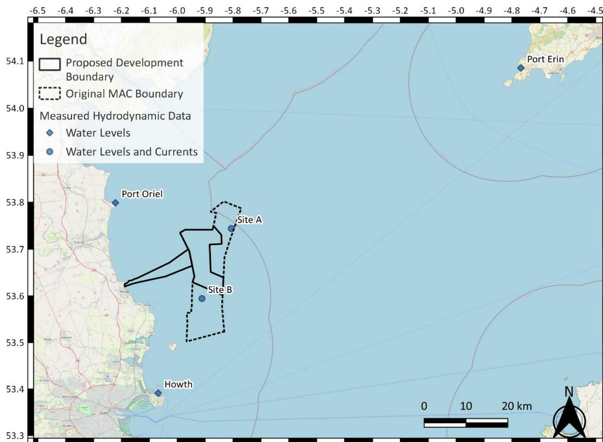
Figure 4.1: Measured datasets considered for hydrodynamic model validation.
