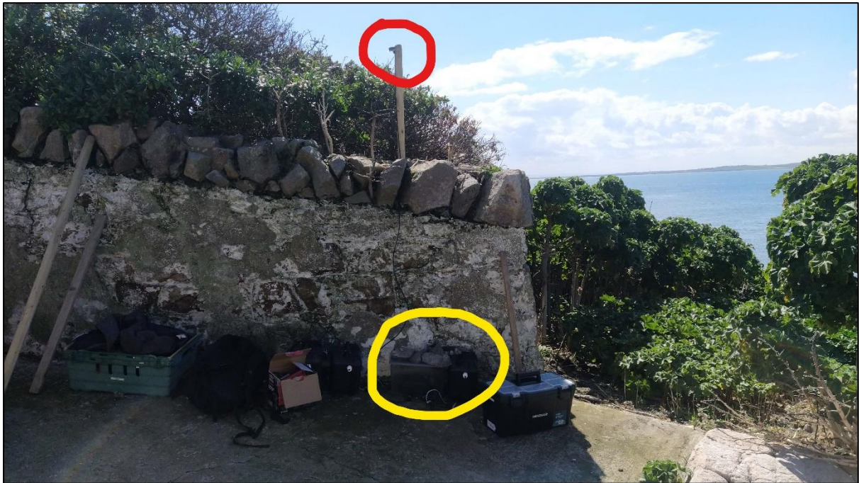
Plate 1 - Western detector, microphone circled in red, detector and battery circled in yellow
