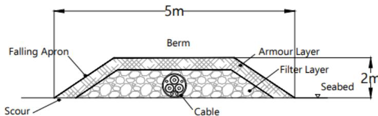
**Image 6.1 Typical Mattress Cable Protection - not to scale (Source: NISA)**
