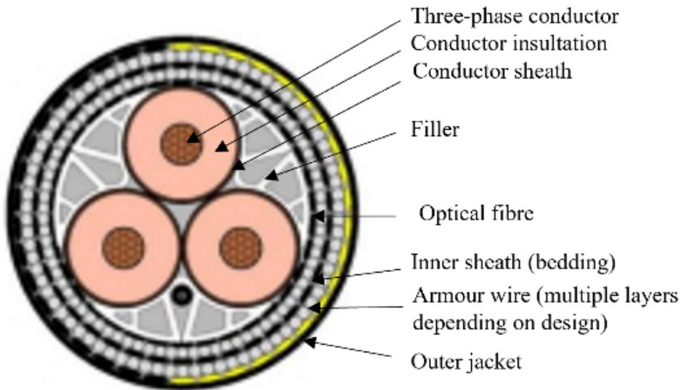
**Image 6.8 Indicative Inter-Array Cable Cross-Section (Source: CIP)**
