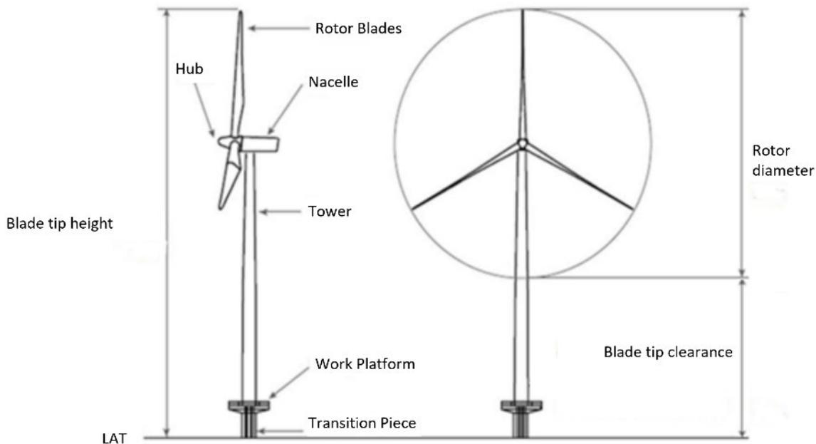
**Image 6.3 Typical WTG Components – not to scale (Source: Arup)**
