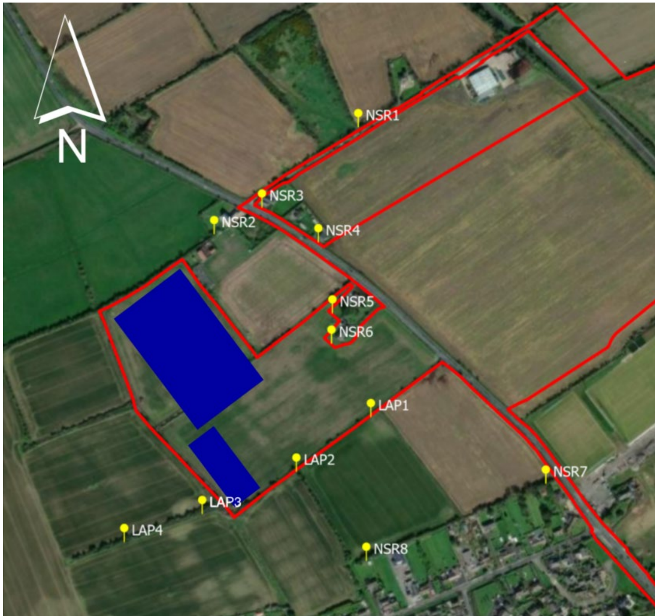
Image A30.3 Noise sensitive receptors (NSRs) in proximity to grid facility and landfall site and the onshore development area shown in red, with approximate footprint of the grid facility shown in dark blue (replaces Table 30.12 in Chapter 30 of the 2024 EIAR)
