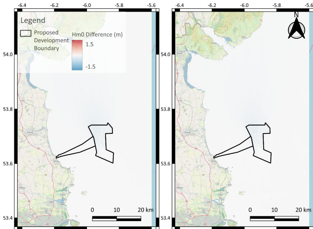
Figure 5.12: Predicted difference in significant wave height due to the imposition of the proposed development during p50 waves from 156°N. Right panel uses present day water level, left panel includes sea level rise.
