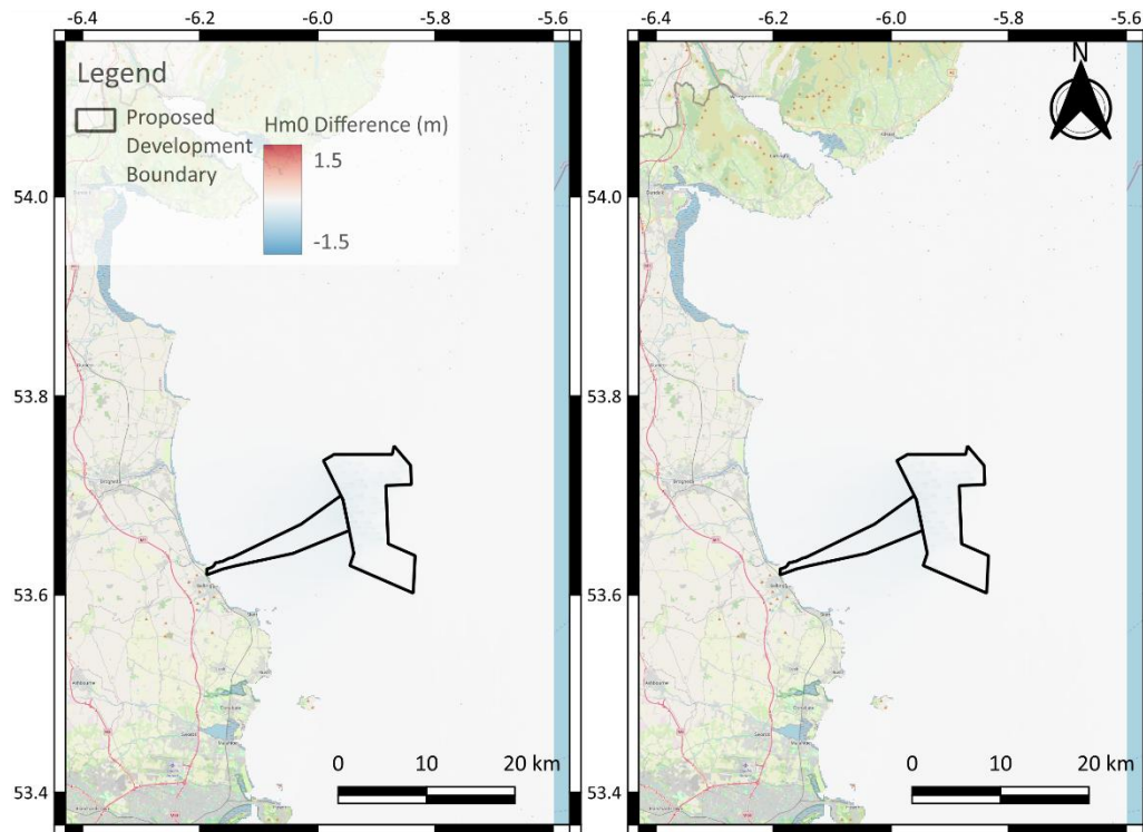
Figure 5.9: Predicted difference in significant wave height due to the imposition of the proposed development during p50 waves from 68°N. Right panel uses present day water level, left panel includes sea level rise.
