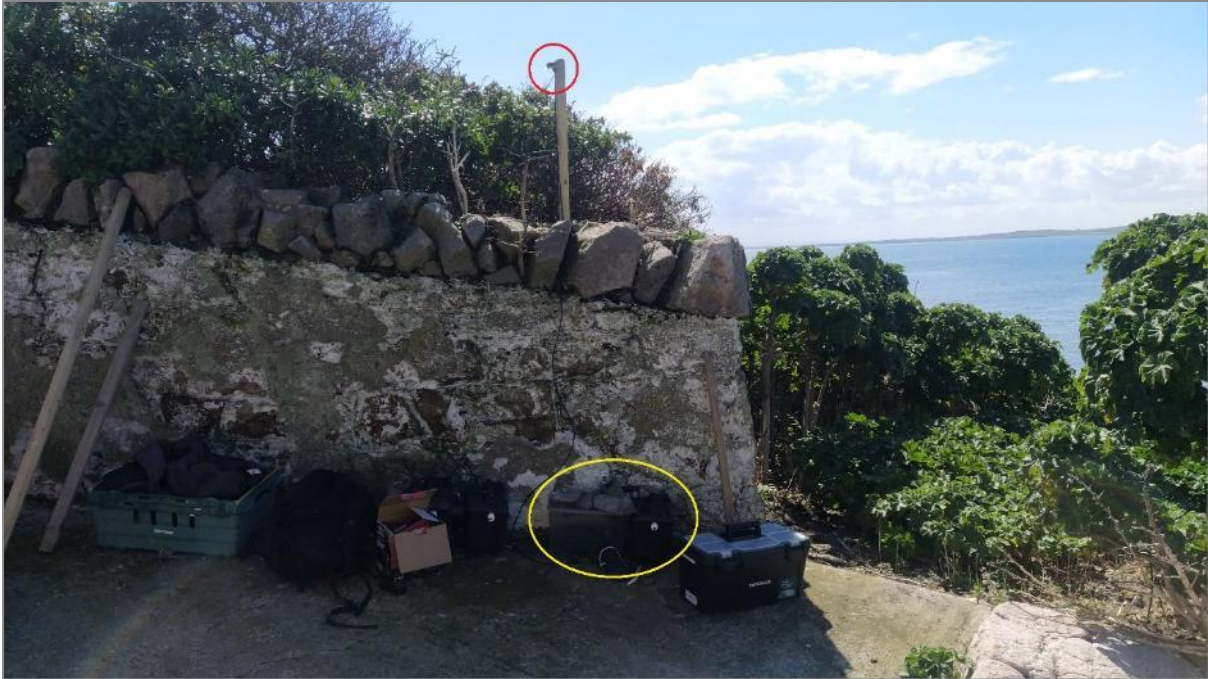
Plate 1: Western detector, microphone circled in red, detector and battery circled in yellow
