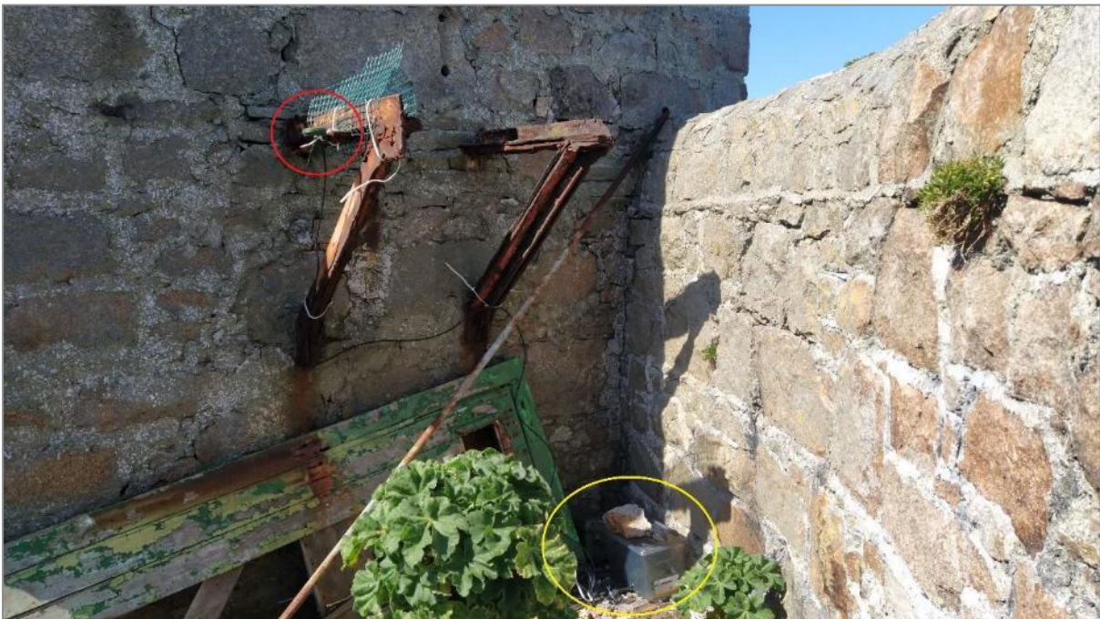
Plate 2: Eastern detector, microphone circled in red, detector and battery circled in yellow.
