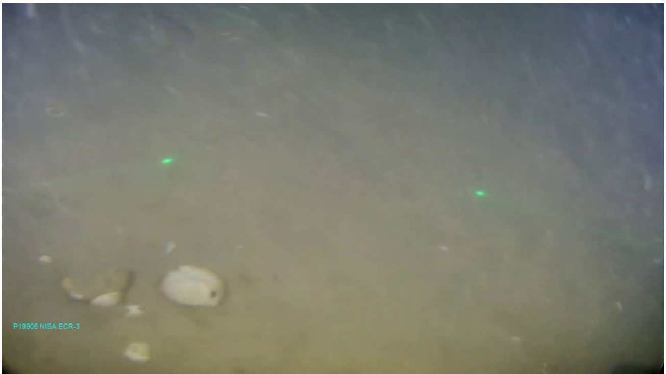
Figure 3.23: ECR-3 – Slightly gravelly muddy sand with shell debris
