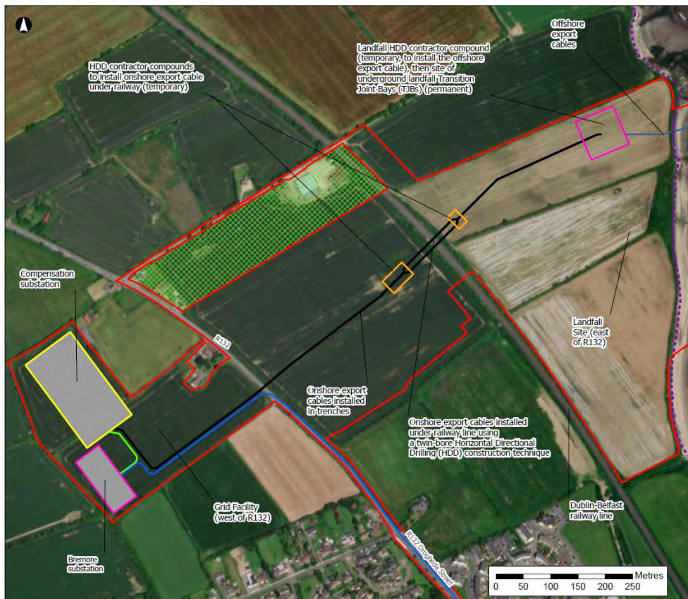
Image 3.3.1 Onshore Infrastructure at Landfall Site and Grid Facility (Figure 7.2 of the 2024 EIAR)
